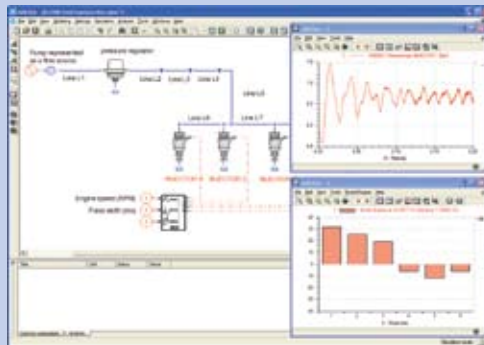
Linear analysis highlights the intrinsic dynamic properties of a gasoline low-pressure injection circuit.
