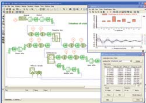
Vibration analysis of a truck driveline: eigenvalues and modal shapes.
