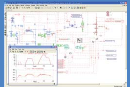
A complete vehicle model including a mean value engine model as the core of an engine HiL test bench.
