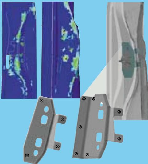
The modified design of the door frame re-reinforcement component improved the total life by a factor exceeding 20.
