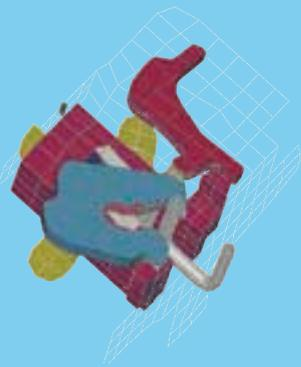
Detailed model of the lock based on a mixture of solid and shell elements.
