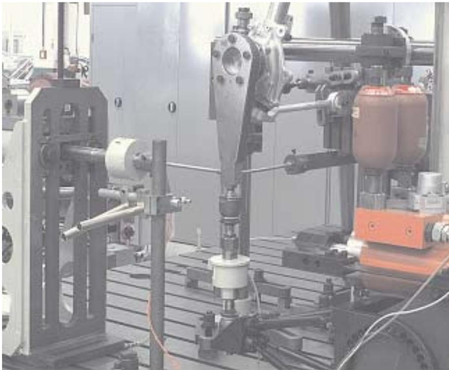
Fig 1: Test rig for the knuckle
