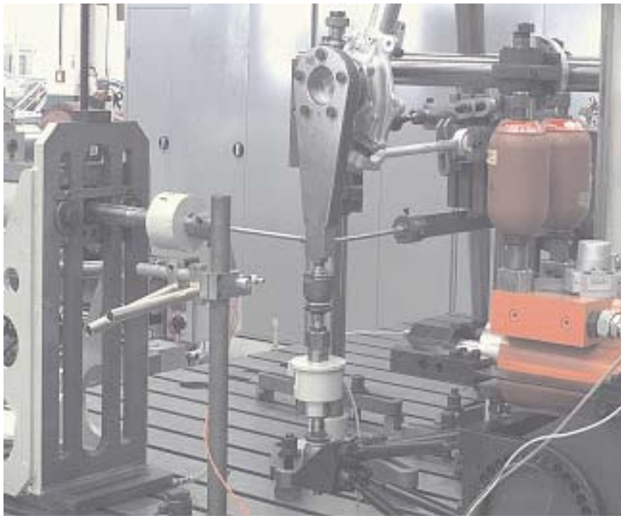
Fig 1: Test rig for the knuckle
