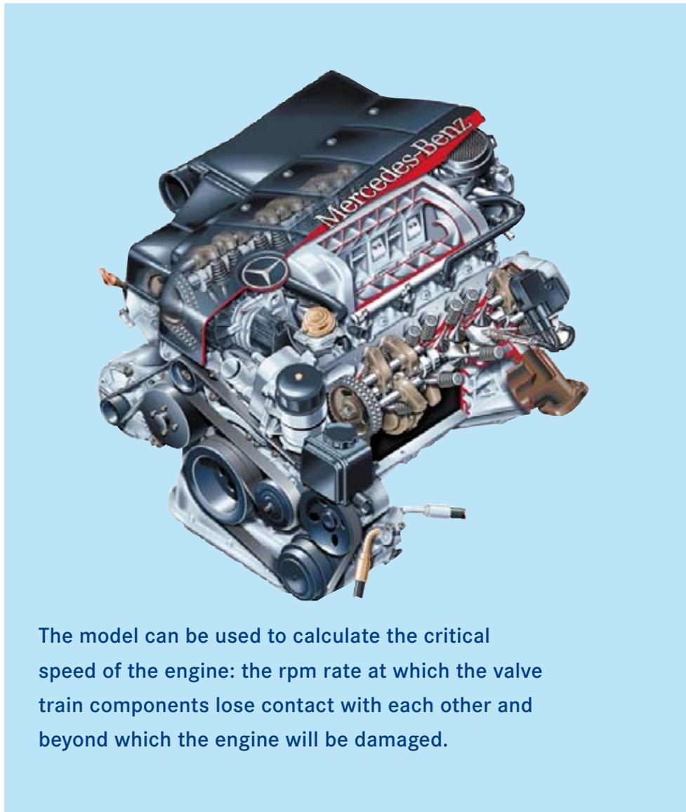
The model can be used to calculate the critical speed of the engine: the rpm rate at which the valve train components lose contact with each other and beyond which the engine will be damaged.
