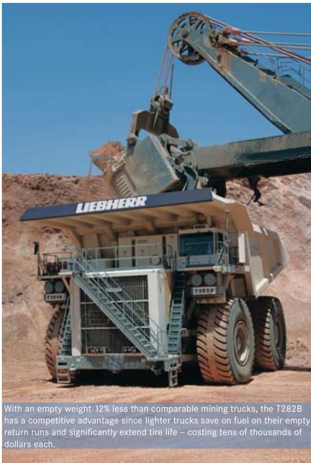
With an empty weight 12% less than comparable mining trucks, the T282B has a competitive advantage since lighter trucks save on fuel on their empty return runs and significantly extend tire life – costing tens of thousands of dollars each.
