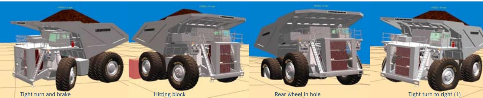
Liebherr analysts used LMS multibody dynamics in studying the behavior of the T282B truck for various load cases including turns, washboarding, braking, acceleration, backing into a barrier and running into holes.
