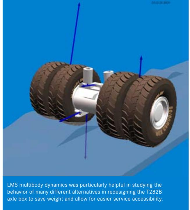
LMS multibody dynamics was particularly helpful in studying the behavior of many different alternatives in redesigning the T282B axle box to save weight and allow for easier service accessibility.
