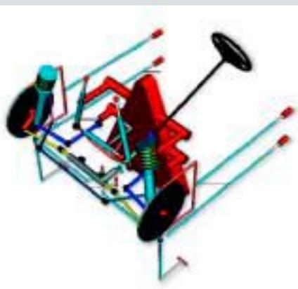
BMW Axle test rig for non-driven front suspensions (left) • BMW Virtual Axle Test Rig model (right)
