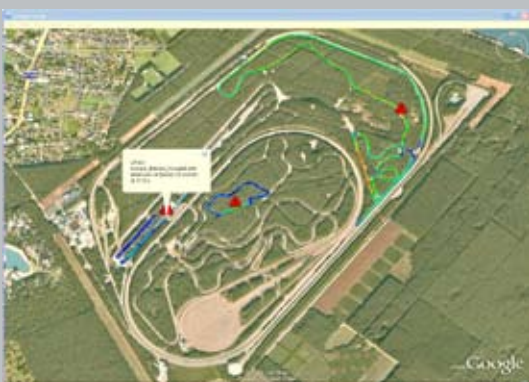
Customer-correlated test schedule by mapping customer usage to proving grounds.
