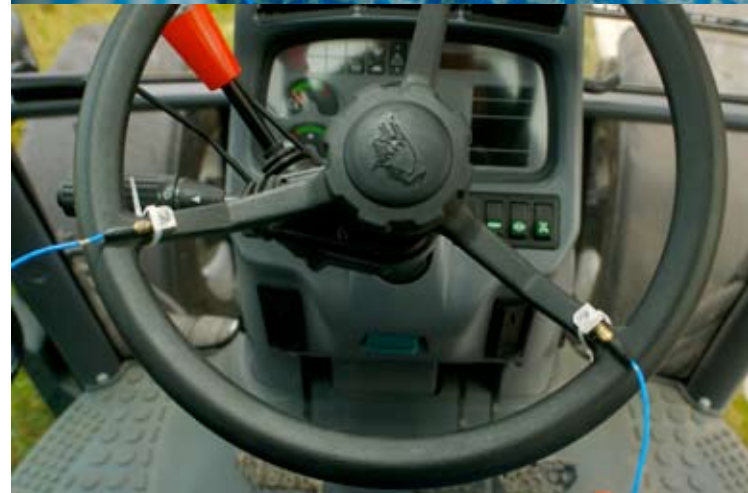
(top) Seat pad sensor to measure seat acceleration in 3 directions (bottom) Mounting of steering wheel accelerometers
