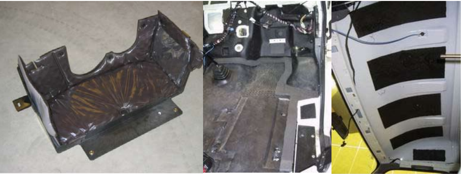
LMS Engineers improved the existing engine undershield and developed a new gearbox undershield to reduce the direct gearbox contributions.
