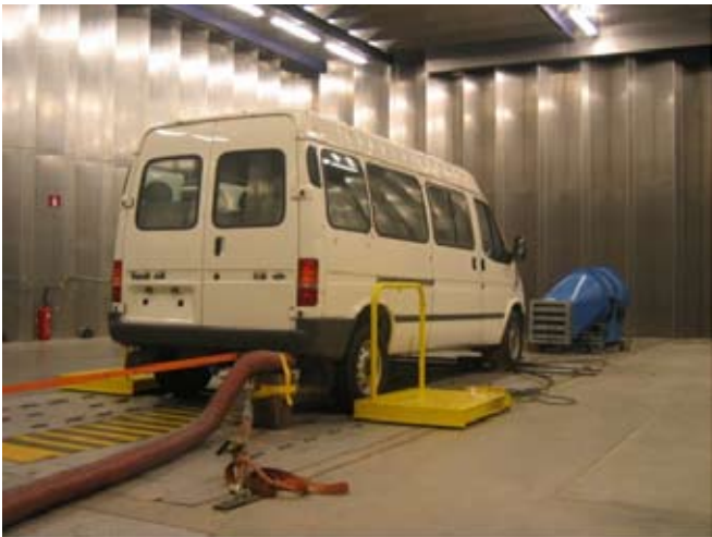
LMS engineers performed extensive indoor pass-by-noise tests on the LMS chassis dyno in the large semi-anechoic room. The advantage of this approach over exterior pass-by-noise measurements is the high repeatability of the measurements and quick setup.
