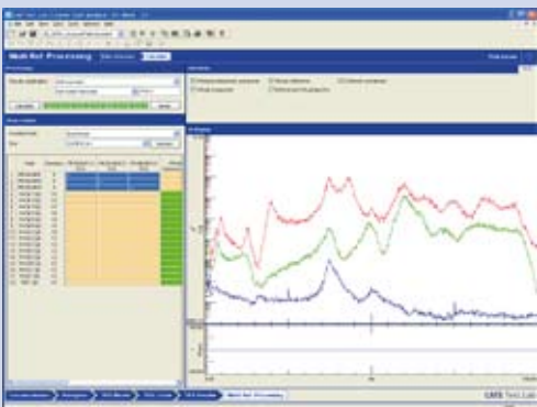
With PCA, engineers decompose the excitation in orthogonal components and select relevant ones.
