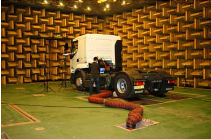
UTAC's vibration and acoustics laboratory is equipped with one of Europe's largest semi-anechoic chambers, which measures 2000 cubic meters. It is equipped with two roller benches for lightweight and heavy-duty vehicles.
